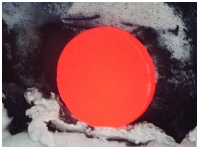
Fig. 4 Image of ZrB_2 -CNT composite with 30 vol% CNT sintered at 1750 °C for 5 min after dynamic heat flux test (sample diameter: 5 cm, sample thickness: 5 mm)
